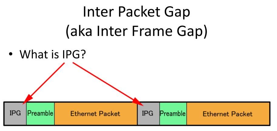
Ethernet devices must allow a minimum idle period between transmission of Ethernet packets. (from wikipedia)
