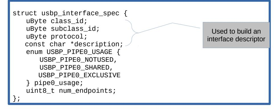
• Used to build a interface descriptor, and to request endpoints to be used for the interface.
